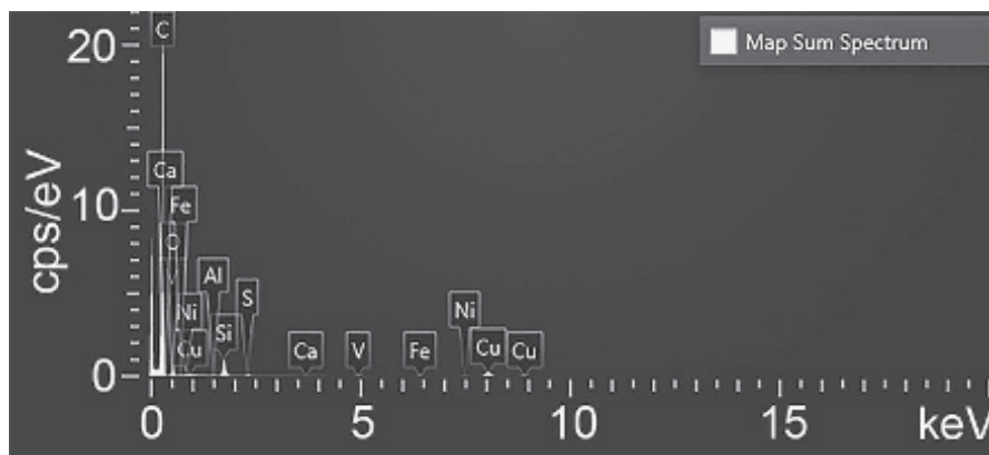
FIGURE 4.30 Energy dispersive X-ray spectrum of hybrid filler Pr/Si 7. (Reprinted from Al-Ghamdi, A. A.; Al-Hartomy, O. A.; Al-Solamy, F. R.; Dishovsky, N.; Mihaylov, M.; Atanasov, N.; Atanasova, G.; Nihtianova, D. Microwave Properties of Natural Rubber Based Composites Comprising Conductive Carbon Black/silica Hybrid Fillers. J. Polym. Res. 2016 , 23, 180. © 2016 With permission of Springer.)
